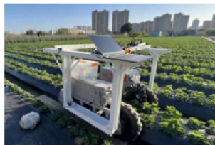
WSU researchers develop an AI robot that uses a puff of air to find and pick ripe strawberries
